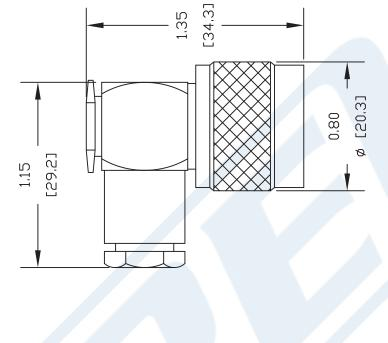
2. FORM BRAID OVER CLAMP NUT (4). CUI DIELECIRIC TO DIMENSION SHOWN. DO NOT NICK CENTER CONDUCTOR. SLIDE ASSEMBLY CONDUCTOR. TIN CENTER CONDUCTOR. SLIDE ASSEMBLY INTO BODY, SOLDER CENTER CONDUCTOR IN PLACE & TIGHTEN CLAMP NUT. SCREW CAP DOWN INTO PLACE.
