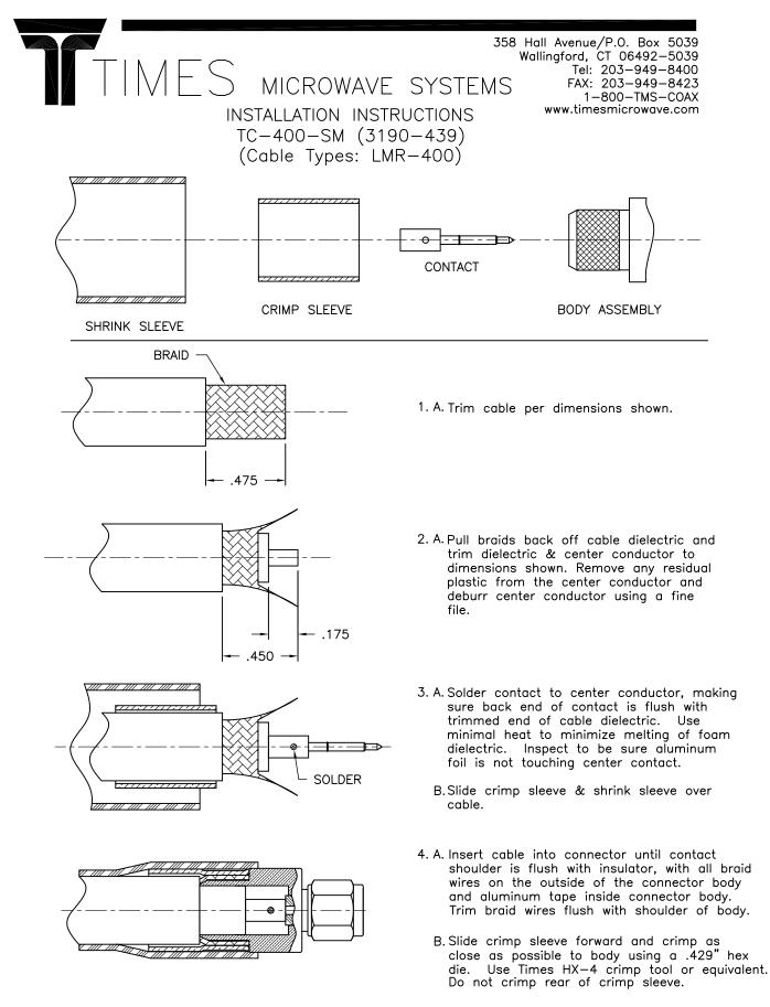
C. Slide shrink sleeve into place and heat shrink over rear of body with hot air gun.
