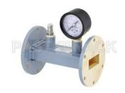
WR-137 Waveguide Pressurizing Section 4.25 Inch Length, UG-344/U Round Cover Flange from 5.85 GHz to 8.2 GHz
