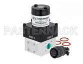
WR-42 Waveguide Electromechanical Relay SPDT Latching Switch, K Band 26.5 GHz Max. Freq., 800 Watts, UG-595/U Square Cover, 12V, TTL
