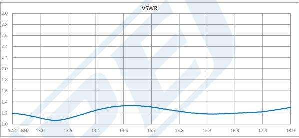
WR-62 UG-419/U Square Cover Flange to SMA Female Waveguide to Coax Adapter Operating from 12.4 GHz to 18 GHz from Pasternack Enterprises has same day shipment for domestic and International orders. Our RF, microwave and millimeter wave products maintain a 99.4% availability and are part of the broadest selection in the industry.
