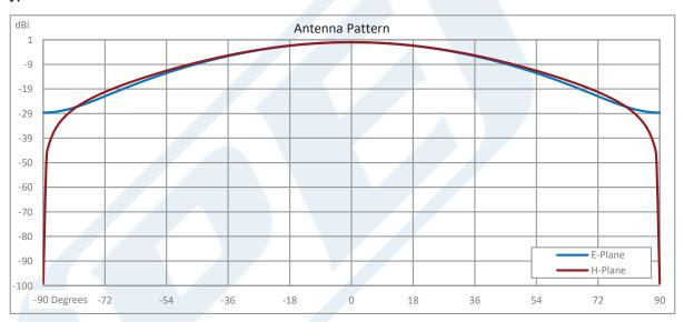
Click the following link (or enter part number in "SEARCH" on website) to obtain additional part information including price, inventory and certifications: WR-10 Waveguide Wide Angle Scalar Feed Horn Antenna Operating from 89 GHz to 99 GHz with a Nominal 10 dBi Gain with UG-385/U-Mod Round Cover PEWAN1074
