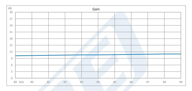
WR-10 Waveguide Wide Angle Scalar Feed Horn Antenna Operating from 89 GHz to 99 GHz with a Nominal 10 dBi Gain with UG-385/U-Mod Round Cover from Pasternack Enterprises has same day shipment for domestic and International orders. Our RF, microwave and millimeter wave products maintain a 99.4% availability and are part of the broadest selection in the industry.
