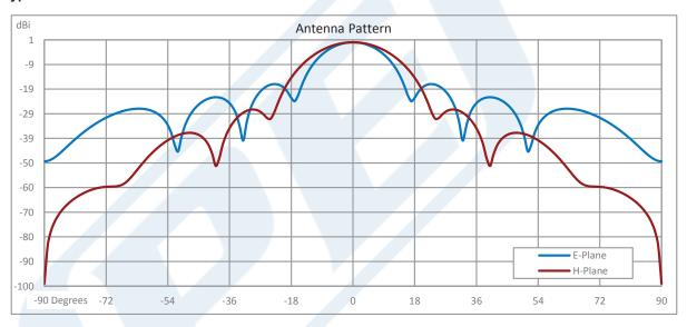
Click the following link (or enter part number in "SEARCH" on website) to obtain additional part information including price, inventory and certifications: WR-6 Waveguide Conical Gain Horn Antenna Operating from 100 GHz to 112 GHz with a Nominal 25 dBi Gain with UG-387/U-Mod Round Cover Flange PEWAN1064
