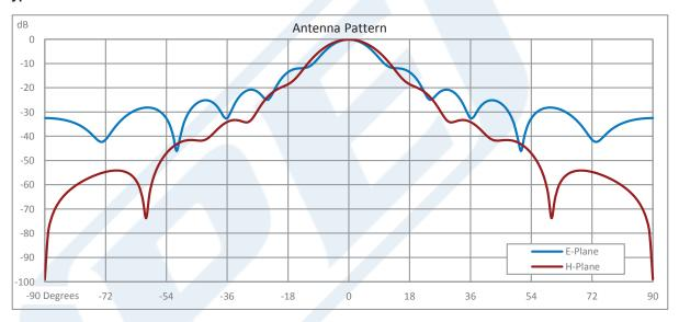
Click the following link (or enter part number in "SEARCH" on website) to obtain additional part information including price, inventory and certifications: WR-6 Waveguide Conical Gain Horn Antenna Operating from 100 GHz to 112 GHz with a Nominal 20 dBi Gain with UG-387/U-Mod Round Cover Flange PEWAN1063
