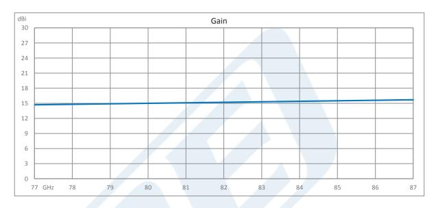
WR-10 Waveguide Conical Gain Horn Antenna Operating from 77 GHz to 87 GHz with a Nominal 15 dBi Gain with UG-387/U Round Cover Flange from Pasternack Enterprises has same day shipment for domestic and International orders. Our RF, microwave and millimeter wave products maintain a 99.4% availability and are part of the broadest selection in the industry.
