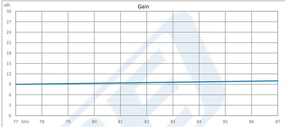
WR-10 Waveguide Conical Gain Horn Antenna Operating from 77 GHz to 87 GHz with a Nominal 10 dBi Gain with UG-387/U Round Cover Flange from Pasternack Enterprises has same day shipment for domestic and International orders. Our RF, microwave and millimeter wave products maintain a 99.4% availability and are part of the broadest selection in the industry.
