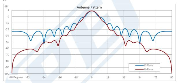
Click the following link (or enter part number in "SEARCH" on website) to obtain additional part information including price, inventory and certifications: WR-10 Waveguide Conical Gain Horn Antenna Operating from 87 GHz to 100 GHz with a Nominal 25 dBi Gain with UG-387/U Round Cover Flange PEWAN1052
