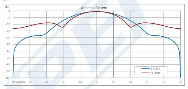
Click the following link (or enter part number in "SEARCH" on website) to obtain additional part information including price, inventory and certifications: WR-12 Waveguide Conical Gain Horn Antenna Operating from 77 GHz to 87 GHz with a Nominal 15 dBi Gain with UG-387/U Round Cover Flange PEWAN1046
