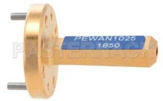
WR-6 Waveguide Standard Gain Horn Antenna Operating from 110 GHz to 170 GHz with a Nominal 10 dBi Gain with UG-387/U-Mod Round Cover Flange
