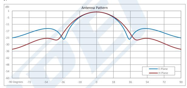
Click the following link (or enter part number in "SEARCH" on website) to obtain additional part information including price, inventory and certifications: WR-12 Waveguide Standard Gain Horn Antenna Operating from 60 GHz to 90 GHz with a Nominal 15 dBi Gain with UG-387/U-Mod Round Cover Flange PEWAN1014
