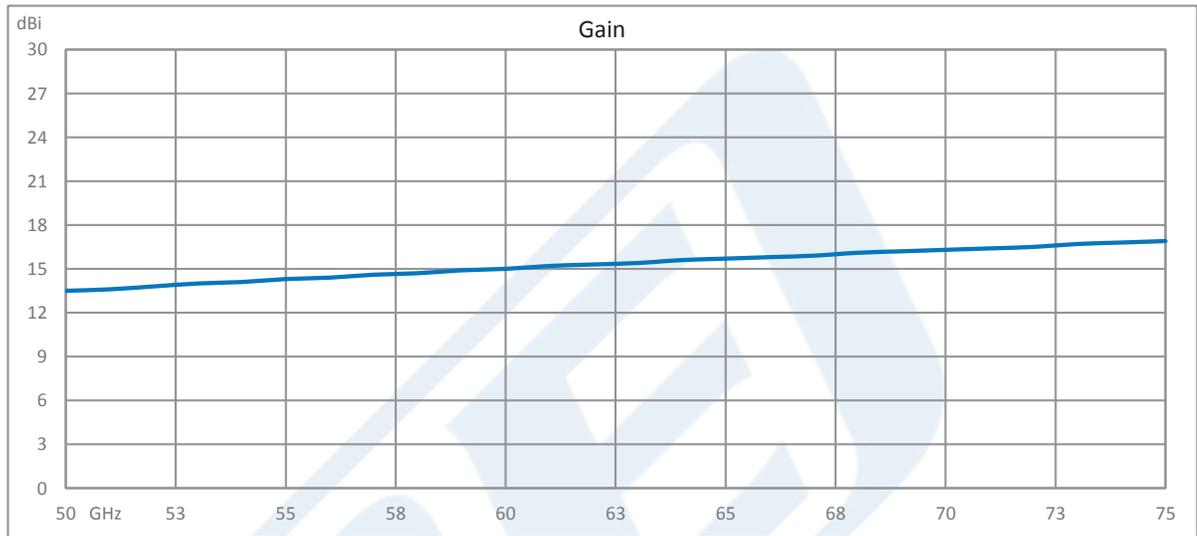
WR-15 Waveguide Standard Gain Horn Antenna Operating from 50 GHz to 75 GHz with a Nominal 15 dBi Gain with UG-385/U-Mod Round Cover Flange from Pasternack Enterprises has same day shipment for domestic and International orders. Our RF, microwave and millimeter wave products maintain a 99.4% availability and are part of the broadest selection in the industry.
