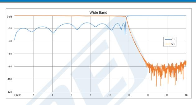
11 Section Lowpass Filter With SMA Female Connectors Operating From DC to 11 GHz from Pasternack Enterprises has same day shipment for domestic and International orders. Our RF, microwave and millimeter wave products maintain a 99.4% availability and are part of the broadest selection in the industry.
