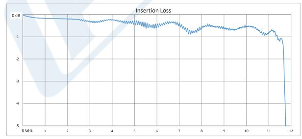
Click the following link (or enter part number in "SEARCH" on website) to obtain additional part information including price, inventory and certifications: 11 Section Lowpass Filter With SMA Female Connectors Operating From DC to 11 GHz PE87FL1017
