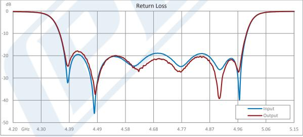
Click the following link (or enter part number in "SEARCH" on website) to obtain additional part information including price, inventory and certifications: 6 Section Bandpass Filter With SMA Female Connectors Operating From 4.4 GHz to 4.95 GHz With a 550 MHz Passband PE8739
