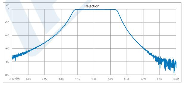
Click the following link (or enter part number in "SEARCH" on website) to obtain additional part information including price, inventory and certifications: 6 Section Bandpass Filter With SMA Female Connectors Operating From 4.4 GHz to 4.95 GHz With a 550 MHz Passband PE8739
