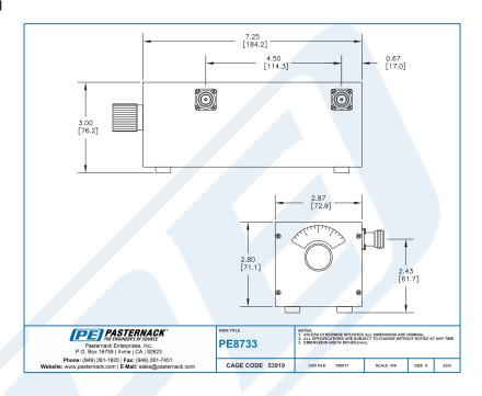
5 Section Tunable Band Pass Filter With N Female Connectors Operating From 1.5 GHz to 3 GHz With a 5% Bandwidth from Pasternack Enterprises has same day shipment for domestic and International orders. Our RF, microwave and millimeter wave products maintain a 99.4% availability and are part of the broadest selection in the industry.
