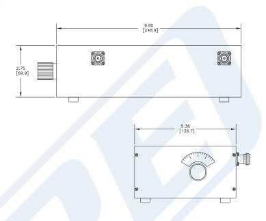
5 Section Tunable Band Pass Filter With N Female Connectors Operating From 750 MHz to 1.5 GHz With a 5% Bandwidth from Pasternack Enterprises has same day shipment for domestic and International orders. Our RF, microwave and millimeter wave products maintain a 99% availability and are part of the broadest selection in the industry.
