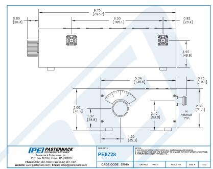
5 Section Tunable Band Pass Filter With N Female Connectors Operating From 125 MHz to 250 MHz With a 5% Bandwidth from Pasternack Enterprises has same day shipment for domestic and International orders. Our RF, microwave and millimeter wave products maintain a 99.4% availability and are part of the broadest selection in the industry.
