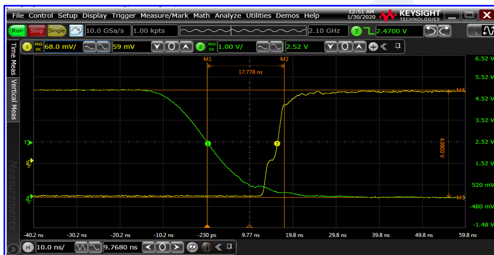
Switching Speed 10 ns Per Div (17.33 ns)
