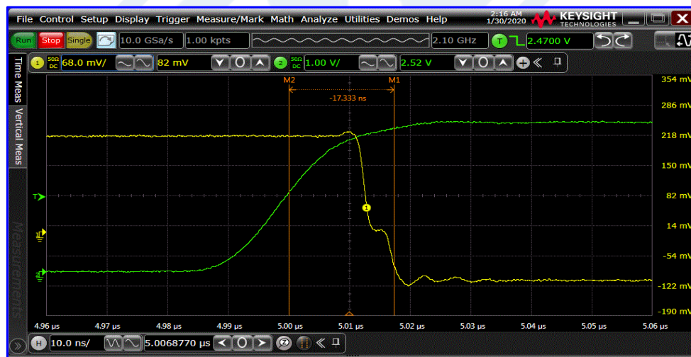
Switching Speed 10 ns Per Div (17.33 ns)
