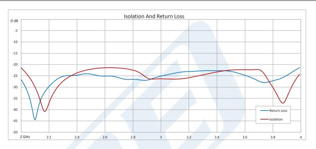
High Power Isolator With 20 dB Isolation From 2 GHz to 4 GHz, 50 Watts And N Female from Pasternack Enterprises has same day shipment for domestic and International orders. Our RF, microwave and millimeter wave products maintain a 99% availability and are part of the broadest selection in the industry.
