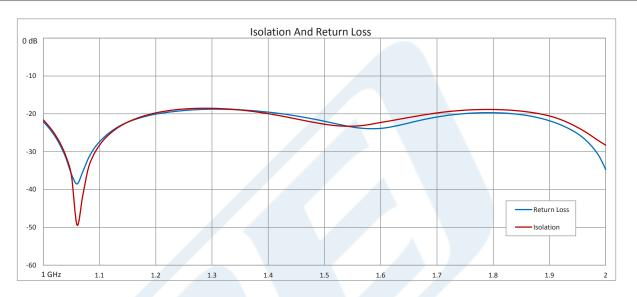
High Power Isolator With 18 dB Isolation From 1 GHz to 2 GHz, 50 Watts And N Female from Pasternack Enterprises has same day shipment for domestic and International orders. Our RF, microwave and millimeter wave products maintain a 99% availability and are part of the broadest selection in the industry.
