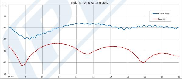
Click the following link (or enter part number in "SEARCH" on website) to obtain additional part information including price, inventory and certifications: Dual Junction Circulator With 32 dB Isolation From 8 GHz to 18 GHz, 5 Watts And SMA Female PE83CR1023
