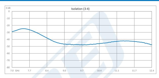
Dual Junction Circulator With 40 dB Isolation From 7 GHz to 12.4 GHz, 5 Watts And SMA Female from Pasternack Enterprises has same day shipment for domestic and International orders. Our RF, microwave and millimeter wave products maintain a 99.4% availability and are part of the broadest selection in the industry.
