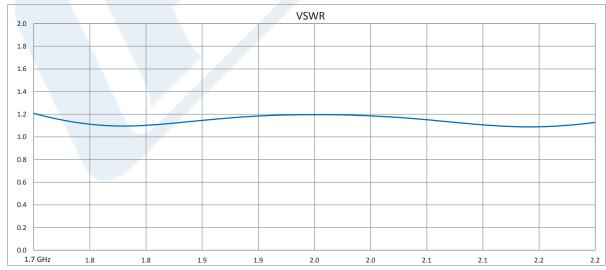
Click the following link (or enter part number in "SEARCH" on website) to obtain additional part information including price, inventory and certifications: Dual Junction Circulator With 40 dB Isolation From 1.7 GHz to 2.2 GHz, 10 Watts And SMA Female PE83CR1015
