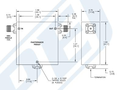
50 Ohm SMA Isolator Operating From 2 GHz to 6 GHz And 25 Watts With 14 dB Isolation from Pasternack Enterprises has same day shipment for domestic and International orders. Our RF, microwave and millimeter wave products maintain a 99% availability and are part of the broadest selection in the industry.
