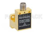
Zero Biased Ka Band Waveguide Detector, WR-28, Negative Video Out, 26.5 GHz to 40 GHz, UG-599/U Square Cover Flange
