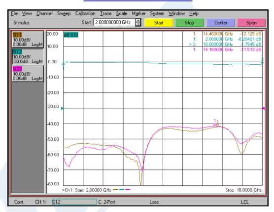
Click the following link (or enter part number in "SEARCH" on website) to obtain additional part information including price, inventory and certifications: SMA High Power Limiter, 200 Watts Peak Power, 100 ns Recovery, 14 dBm Flat Leakage, 2 GHz to 18 GHz PE80L3000
