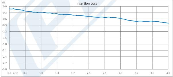
Click the following link (or enter part number in "SEARCH" on website) to obtain additional part information including price, inventory and certifications: High Power Limiter, Field Replaceable SMA, 100W Peak Power, 15 us Recovery, 13 dBm Flat Leakage, 20 MHz to 4 GHz PE80L2003
