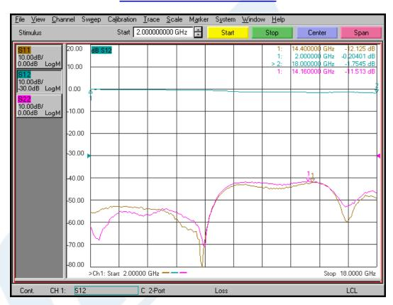
Click the following link (or enter part number in "SEARCH" on website) to obtain additional part information including price, inventory and certifications: SMA High Power Limiter, 200 Watts Peak Power, 100 ns Recovery, 14 dBm Flat Leakage, 2 GHz to 18 GHz PE80L2001
