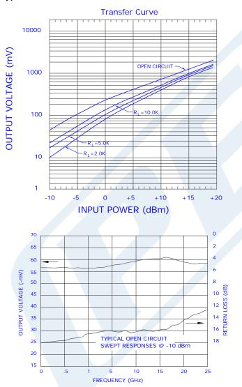
Click the following link (or enter part number in "SEARCH" on website) to obtain additional part information including price, inventory and certifications: Schottky Zero Bias Detector, SMA, Negative Video Out, +20 dBm max Pin, 10 MHz to 12.4 GHz PE8012
