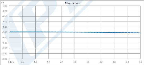
Click the following link (or enter part number in "SEARCH" on website) to obtain additional part information including price, inventory and certifications: 6 dB Fixed Attenuator, QMA Male to QMA Female Brass Tri-Metal Body Rated to 1 Watt Up to 6 GHz PE7AP1002-6
