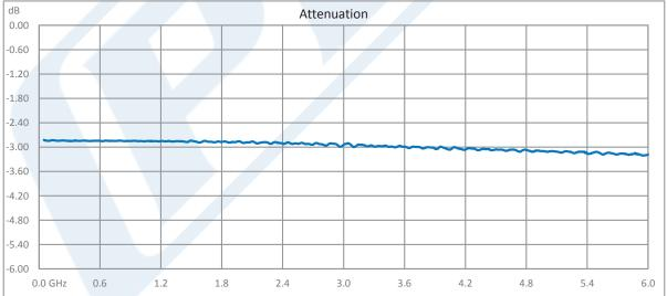
Click the following link (or enter part number in "SEARCH" on website) to obtain additional part information including price, inventory and certifications: 3 dB Fixed Attenuator, QMA Male to QMA Female Brass Tri-Metal Body Rated to 1 Watt Up to 6 GHz PE7AP1002-3
