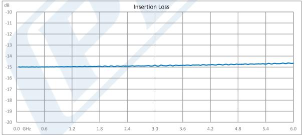
Click the following link (or enter part number in "SEARCH" on website) to obtain additional part information including price, inventory and certifications: 15 dB Fixed Attenuator, QMA Male to QMA Female Brass Tri-Metal Body Rated to 1 Watt Up to 6 GHz PE7AP1002-15
