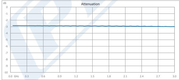
Click the following link (or enter part number in "SEARCH" on website) to obtain additional part information including price, inventory and certifications: 3 dB Fixed Attenuator, QN Male to QN Female Brass Tri-Metal Body Rated to 1 Watt Up to 3 GHz PE7AP1000-3
