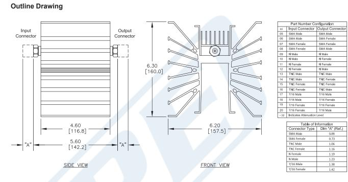
30 dB Fixed Attenuator, TNC Male To TNC Male Directional Black Aluminum Heatsink Body Rated To 300 Watts Up To 3 GHz from Pasternack Enterprises has same day shipment for domestic and International orders. Our RF, microwave and millimeter wave products maintain a 99% availability and are part of the broadest selection in the industry.
