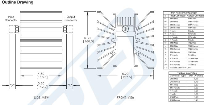
3 dB Fixed Attenuator, SMA Female To SMA Female Directional Black Aluminum Heatsink Body Rated To 300 Watts Up To 3 GHz from Pasternack Enterprises has same day shipment for domestic and International orders. Our RF, microwave and millimeter wave products maintain a 99% availability and are part of the broadest selection in the industry.
