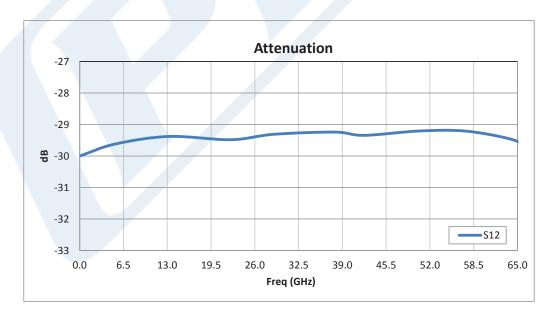
Click the following link (or enter part number in "SEARCH" on website) to obtain additional part information including price, inventory and certifications: 30 dB Fixed Attenuator, 1.85mm Male to 1.85mm Female Passivated Stainless Steel Body Rated to 1 Watt Up to 65 GHz PE7403-30
