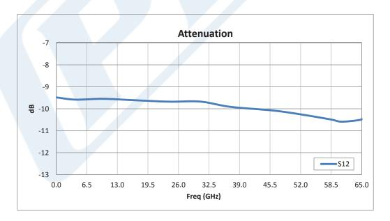
Click the following link (or enter part number in "SEARCH" on website) to obtain additional part information including price, inventory and certifications: 10 dB Fixed Attenuator, 1.85mm Male to 1.85mm Female Passivated Stainless Steel Body Rated to 1 Watt Up to 65 GHz PE7403-10
