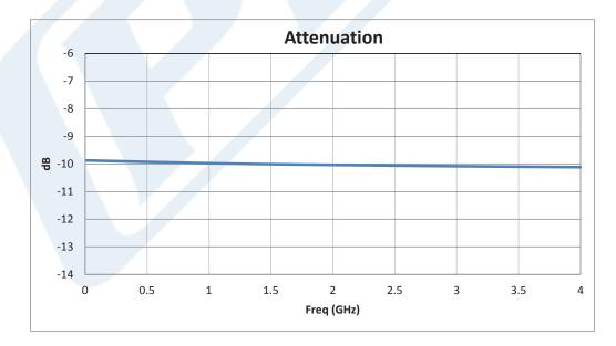
Click the following link (or enter part number in "SEARCH" on website) to obtain additional part information including price, inventory and certifications: 10 dB Fixed Attenuator, SMA Male to SMA Female Black Anodized Aluminum Heatsink Body Rated to 25 Watts Up to 4 GHz PE7393-10
