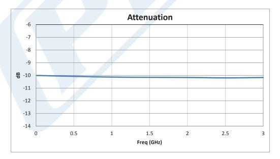
Click the following link (or enter part number in "SEARCH" on website) to obtain additional part information including price, inventory and certifications: 10 dB Fixed Attenuator, SMA Male to SMA Female Aluminum Body Rated to 5 Watts Up to 3 GHz PE7391-10
