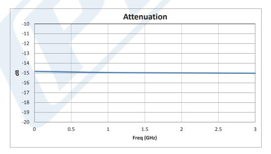
Click the following link (or enter part number in "SEARCH" on website) to obtain additional part information including price, inventory and certifications: 15 dB Fixed Attenuator, N Male to N Female Aluminum Body Rated to 5 Watts Up to 3 GHz PE7390-15
