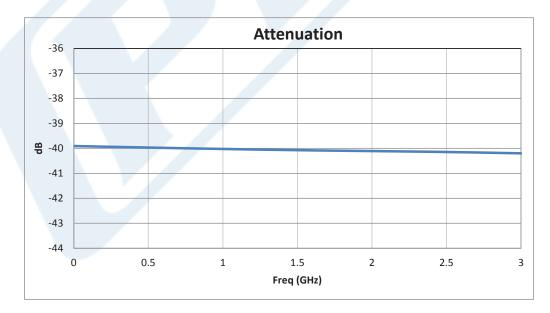
Click the following link (or enter part number in "SEARCH" on website) to obtain additional part information including price, inventory and certifications: 40 dB Fixed Attenuator, N Male to N Female Black Anodized Aluminum Heatsink Body Rated to 50 Watts Up to 3 GHz PE7389-40
