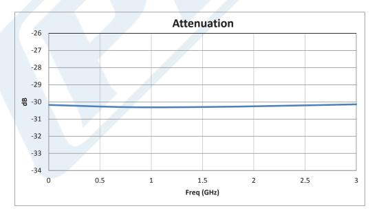
Click the following link (or enter part number in "SEARCH" on website) to obtain additional part information including price, inventory and certifications: 30 dB Fixed Attenuator, N Male to N Female Black Anodized Aluminum Heatsink Body Rated to 50 Watts Up to 3 GHz PE7389-30
