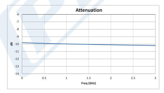
Click the following link (or enter part number in "SEARCH" on website) to obtain additional part information including price, inventory and certifications: 10 dB Fixed Attenuator, N Male to N Female Black Anodized Aluminum Heatsink Body Rated to 50 Watts Up to 3 GHz PE7389-10
