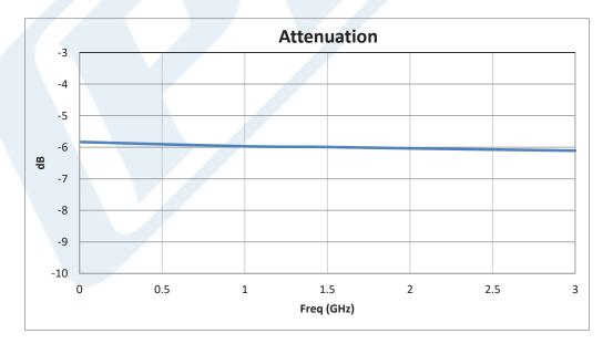
Click the following link (or enter part number in "SEARCH" on website) to obtain additional part information including price, inventory and certifications: 6 dB Fixed Attenuator, N Male To N Female Unidirectional Black Anodized Aluminum Heatsink Body Rated To 50 Watts Up To 3 GHz PE7388-6
