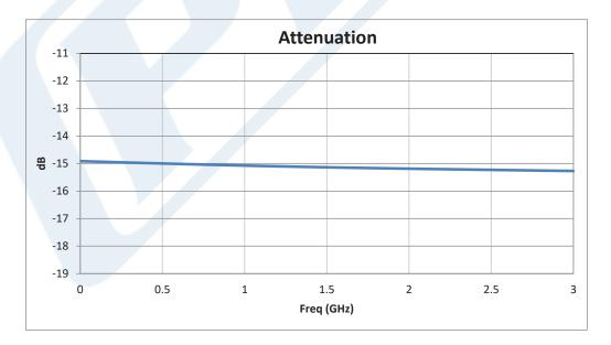
Click the following link (or enter part number in "SEARCH" on website) to obtain additional part information including price, inventory and certifications: 15 dB Fixed Attenuator, N Male To N Female Unidirectional Black Anodized Aluminum Heatsink Body Rated To 50 Watts Up To 3 GHz PE7388-15
