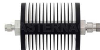
10 dB Fixed Attenuator, SMA Male to TNC Female Black Anodized Aluminum Heatsink Body Rated to 25 Watts Up to 18 GHz
