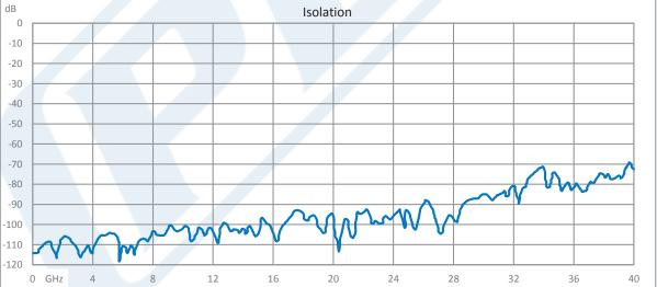
Click the following link (or enter part number in "SEARCH" on website) to obtain additional part information including price, inventory and certifications: SP4T 0.05 dB Low Insertion Loss Repeatability Relay Latching Switch, Terminated, DC to 40 GHz, 5W, 24V, Indicators, Self Cut Off, 2.92mm PE71S6334
